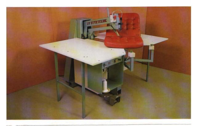
The HECTOR presses the cushion together at the tufting point and sews a pattern, which provides an everlasting compression of the cushion and keeps the fabric and filling in place.
